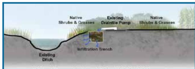
Typical cross section trench concept
